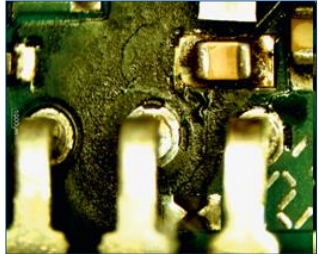
Electronic migration on an electronic assembly group (Source: AUCOTEAM GmbH)
